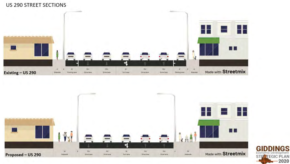
FIGURE 5.3: US-290 STREET SECTIONS (EXISTING VS. PROPOSED)
